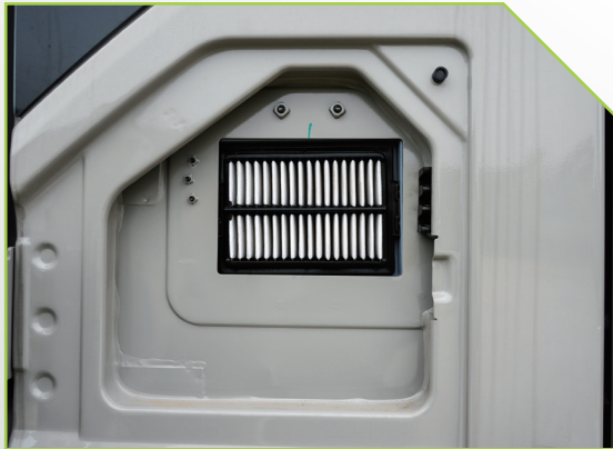
Engine fuel filters, oil filter, air cleaner, hydraulic oil pilot filter and A/C filter are easily accessible at ground level, achieving "one-stop" maintenance on the ground.
