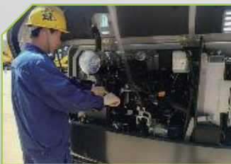
燃油滤和机油滤保养 Maintenance of fuel filters and engine oil filter
