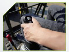
Adjustable armrest, which perfectly matches with the joystick, letting the operator work in the most comfortable posture with high efficiency.
