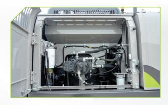
The inspection and maintenance of the oil filter, diesel filter and pilot filter are all within easy reach, realizing one-stop mainte-
