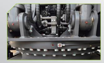
Added with the centralized lubrication function of the slewing bearing to make maintenance more convenient.
