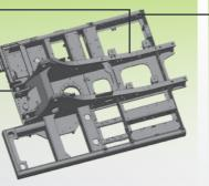
The side beams are upgraded from C-shaped beams to D-shaped beams, and a stronger upper frame structure,compared with the previous generation model, the cross-sectional area is improved by 37%, and the strength is improved
