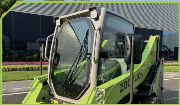
FOPS/ROPS cab A FOPS/ROPS certified cab provides protection in the event of unforeseen rollovers and falling objects.
