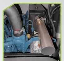
Integral muffler structure, lowering vibration and noise Air inlet of muffler is connected with the engine exhaust out let directly.
