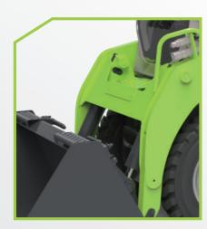
• Bucket cylinders and pipelines are equipped with protective cover to prevent them from being damaged.
