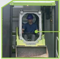
• Hydraulic pilot controlling technology making it easy for drivers to control with only 1/3 control force of mechanical control
