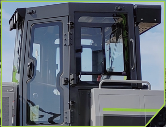
Sealed cabin with special-shaped frame 异型材骨架密封驾驶室
