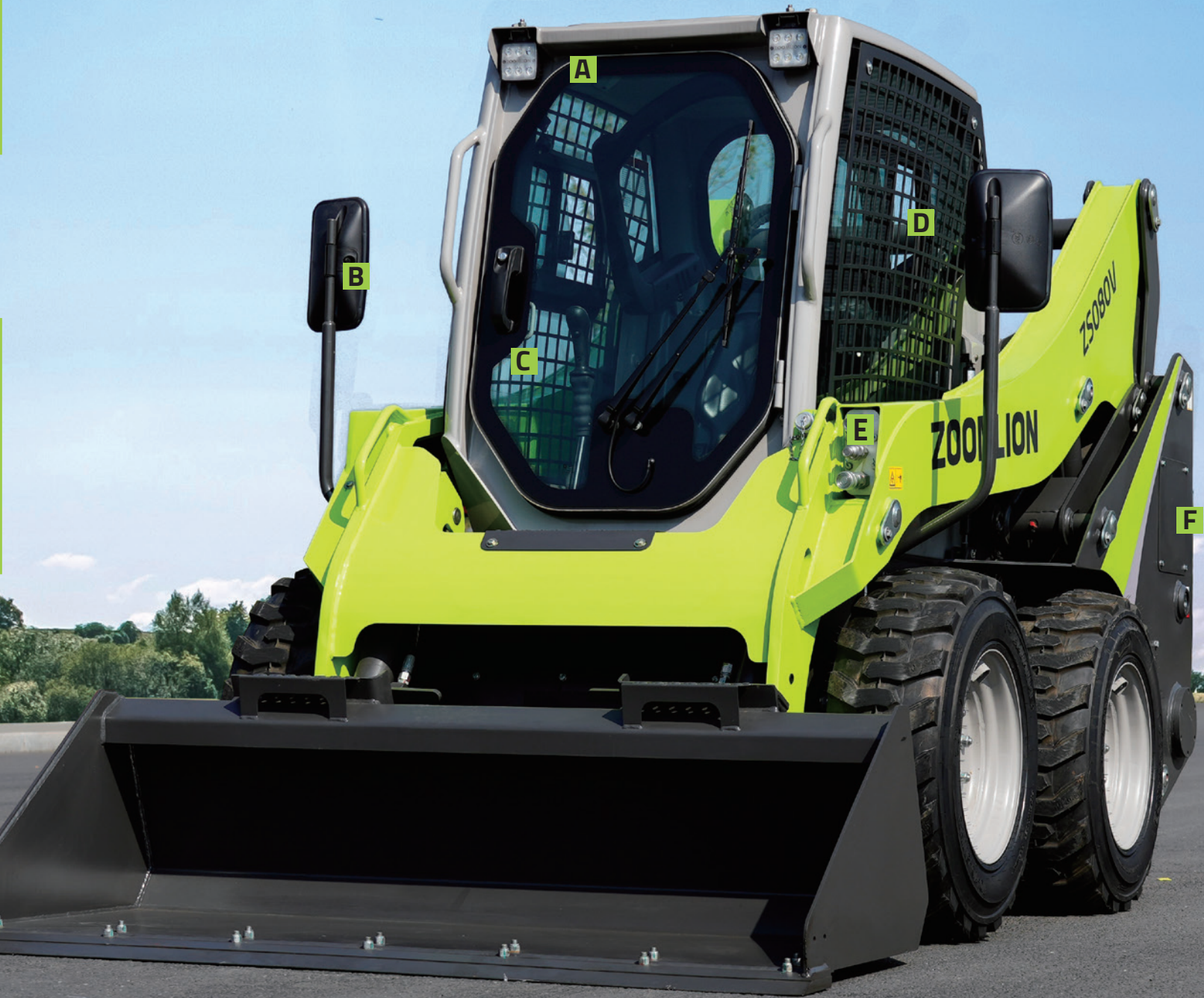
Optional turn signals and exterior rearview mirrors 可选转向灯和车外后视镜
