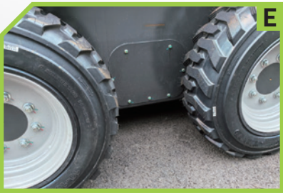
Side-mounted sprocket box 侧置链轮箱
