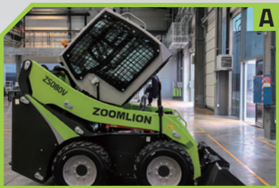
Interior maintenance 内部维护
