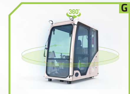
Superb all-round visibility thanks to large window areas, with increased glass transmittance above 11% Standard sunshade 大面积环绕式玻璃玻璃通透率提升11%以上 标配遮阳帘
