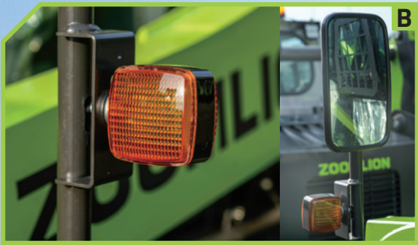
Optional turn signals and exterior rearview mirrors They do not move with the lift arm, making it easy to observe the situation at the back of the body at any time and keeping you safe.
