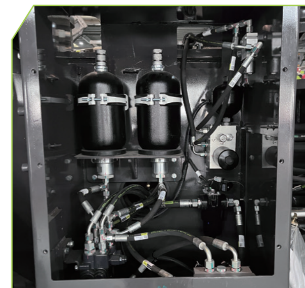
The pilot filter and brake filter are centrally arranged on the right side, within easy reach for maintenance and convenience.
