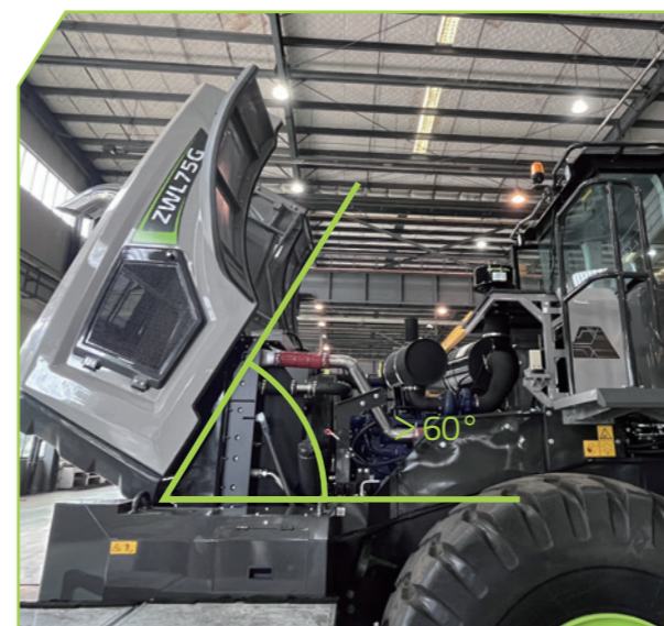
The engine hood can tilt backward by more than 60^\circ , providing convenient maintenance, repair and inspection for internal filters with a large service space.
