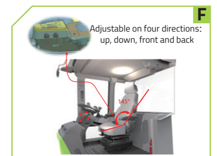
Spacious operating space, adjustable armrest box and handle, providing a more comfortable driving experience.
