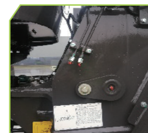
Grease lubrication points are centrally led out for ground-level access, enabling convenient daily maintenance.
