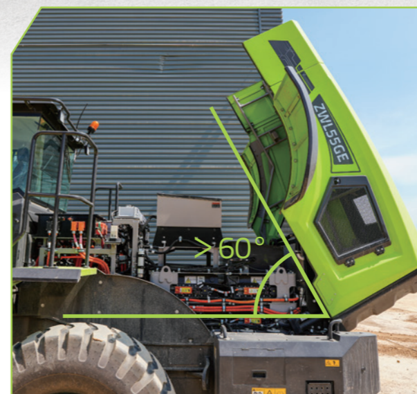
The engine hood can tilt backward by more than 60°, providing convenient maintenance, repair and inspection for internal filters with a large service space.
