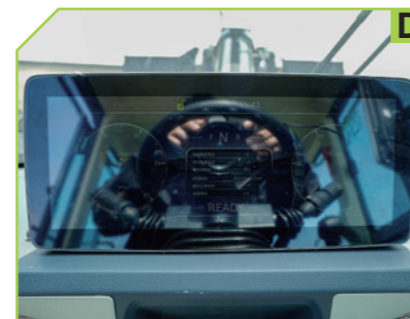
1. 12.3-inch LCD dashboard 2. Equipped with fault detection and fault codes display.
