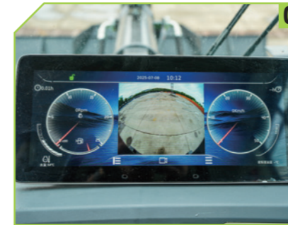
12.3-inch LCD touch-screen monitor, with standard back-up camera; Equipped with fault detection and fault codes display.
