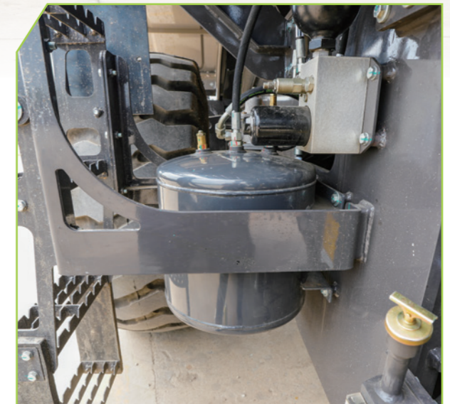
The tank bodies are arranged centrally, accessible from the ground, making daily maintenance convenient.
