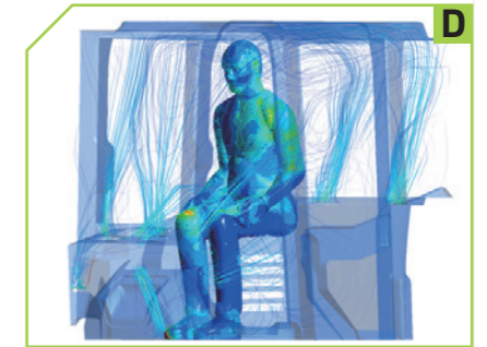
The cab is hermetically sealed with a pressure of +50 Pa, and equipped with N95-class filter elements, with a PM2.5 filtration efficiency of ≥99%
