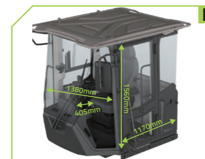
With 360° large-area panoramic glass stretching to the floor, the vision area reaches 3.52 m 2 , the largest in the industry, ensuring extremely broad operational visibility.
